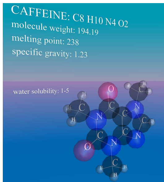
Figure 2. Result of the basic CML2X3D transformation. XSLT stylesheet 1 produces a visualization of the molecular structure with a fixed transparency and the related compound information is shown on an arbitrary plane behind the furthest atom with a default font.
